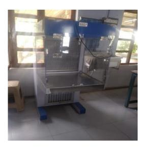
The Laminar Air Flow unit "MO-MODE Aircon 711817DEL" is designed to create a clean and sterile working environment by directing a continuous stream of filtered air in a laminar flow pattern. Laminar flow refers to the smooth, unidirectional airflow that minimizes the presence of airborne contaminants such as dust, particles, and microorganisms.
