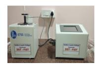
The Paar Solutions Calorimeter, also known as a bomb calorimeter, is a device used to measure the heat of combustion or calorific value of a sample. It works by burning a sample in a high-pressure oxygen environment and measuring the resulting heat release. The calorimeter is typically equipped with a Thermometer, which is used to monitor the temperature changes during the combustion process.
