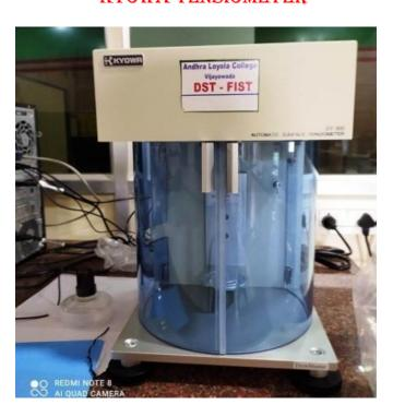
The Kyowa Tensiometer is a device used to measure the surface tension of liquids, which is a crucial parameter in various fields such as chemistry, physics, materials science, and biology. Surface tension is the force acting along the surface of a liquid that tends to minimize its surface area, resulting in behaviors like capillary action, droplet formation, and wetting properties
