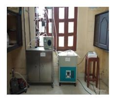
The VLE (Vapor-Liquid Equilibrium) Apparatus with Borosilicate glass components, operating at 0.1 atm and 0°C temperature, typically consists of a temperature bath made of SS304 stainless steel and a vacuum pump such as the UPERFIT Model 50-D.
