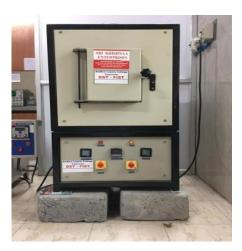
The High Temperature Box Furnace from KE is a muffle furnace capable of reaching temperatures up to 1600°C. Muffle furnaces are commonly used in laboratories and industrial settings for high-temperature applications such as heat treatment, ashing, calcination, sintering, and material testing.
