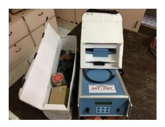
The OMEGA & GM Counting System Model GS-602-A is a gamma-ray spectrometer and gamma-ray counter system used in nuclear science and radiation measurement applications. It is designed to detect and analyze gamma radiation emitted by radioactive isotopes or sources.
